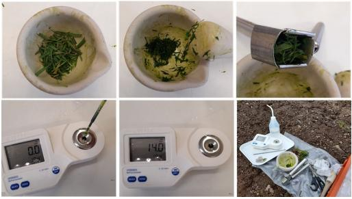
**Figure 4.2**. Measuring leaf nutritional health using a BRIX meter. From top left to right: Cut lengths from several leaves into a mortar (bowl) and grind with a pestle; place sample into a garlic crusher to extract a few drops of sap. From bottom leaft to right: Pipette 2 drops of sap into refractometer cell. The zero reading is calibrated with water. In this example the BRIX reading is 14.0.
